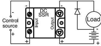
Examples of fast-recovery diodes that may be used for transient suppression:
