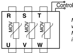
Model RS\_A-660-30-3D0 shown with customer-installed MOVs. Model RS\_A-560-30-3D2 has 3 internal MOVs installed
