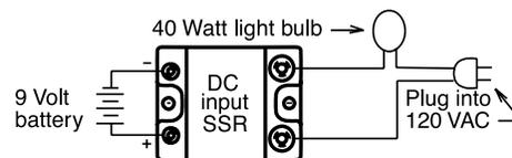
Solid State Relays are NOT open circuits, even when in the off-state, due to their leakage current. Safety can only be achieved by a mechanical disconnect between the solid state relay and the power lines.
