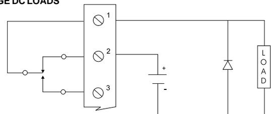
Use a diode with a reverse breakdown voltage two to three times the circuit voltage and forward current at least as large as the load current.
