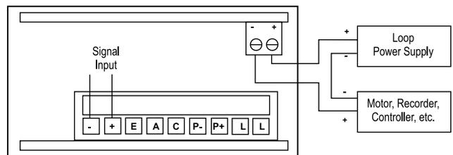
4-20mA output signal being powered from an external 24V power supply.
