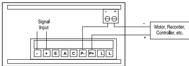
4-20mA output signal being powered by V430's internal 24V power supply. (AC powered units only)
